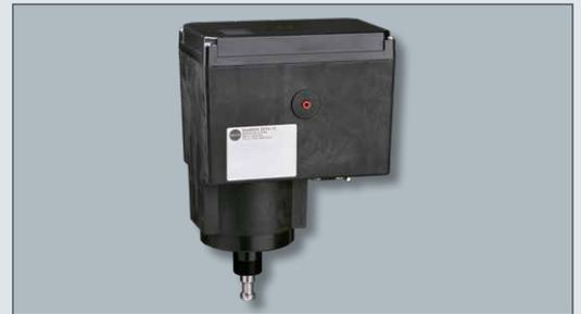
**Types 5857/5827** – Even these „small“ SAMSON actuators come with a huge range of functions. It takes but a few steps to mount them on the valve with a force-locking or form-fit connection. The versions with integrated positioner include automatic calibration to the valve, blocking protection, and further actuator functions that can be customized using the TROVIS-VIEW software.
