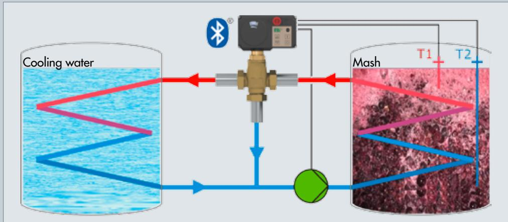
Fixed set point control with mean value calculation, pump control, and set point adjustment at the device
