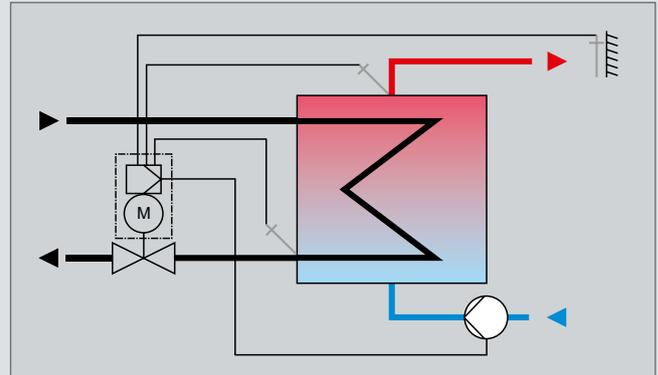
Flow temperature control based on the outdoor temperature with return flow temperature limitation and pump control
