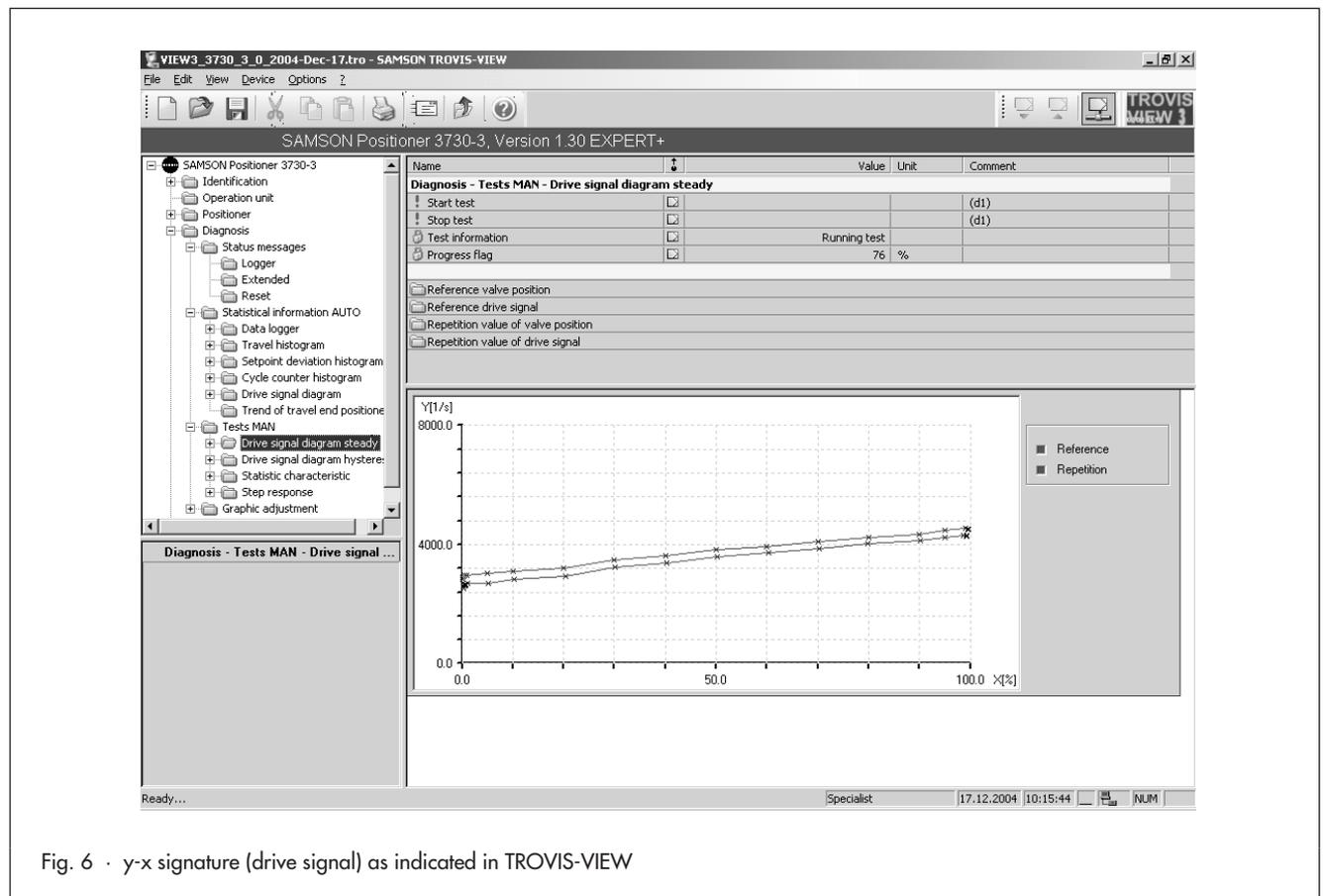
Fig. 6 · y-x signature (drive signal) as indicated in TROVIS-VIEW
