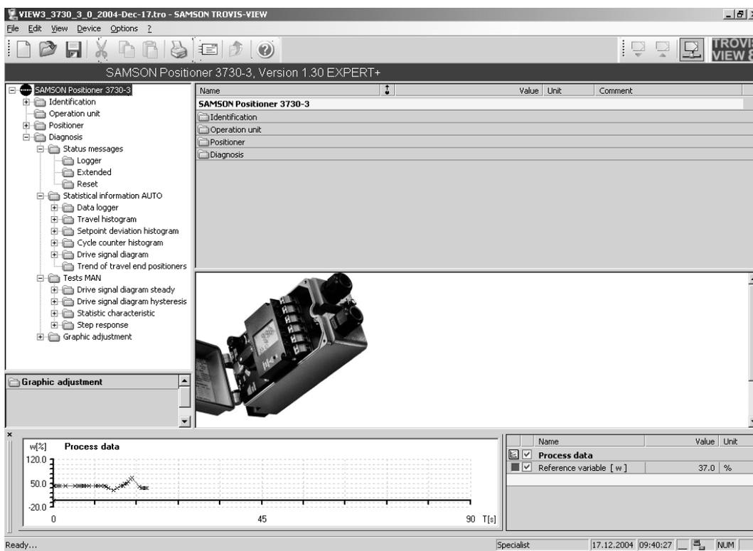
Fig. 3 · TROVIS-VIEW, graphical user interface with Type 3730-3 Positioner
