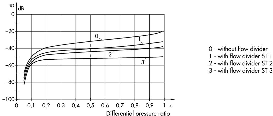
Diagram 1: Noise reduction with gases depending on the differential pressure using flow dividers
