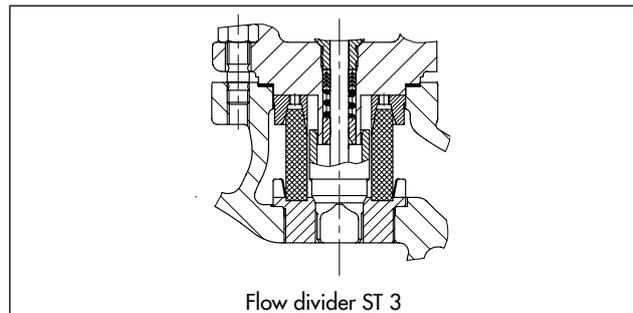
The valve-specific correction values for gases and vapors are required for noise calculation according to VDMA 24422, Edition 1989 and IEC 60534 when flow dividers are used. Refer to the diagrams in section 'Calculation of noise emission' for details.
