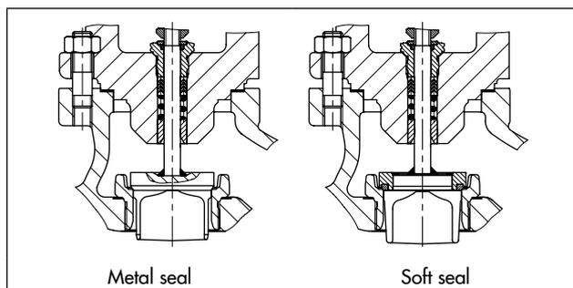
The seat, plug and plug stem are made of stainless steel. In some cases, the trims are subject to high stress due to high differential pressures, cavitation, flashing or in cases where the process media contains solids. In order to increase the service life, seats and metal-seated plugs can have a Stellite® facing and plugs up to DN 100 can be made of solid Stellite®.
