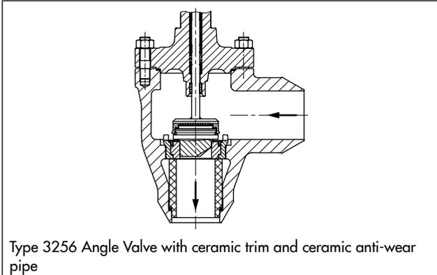
Type 3256 Angle Valve with ceramic trim and ceramic anti-wear pipe
