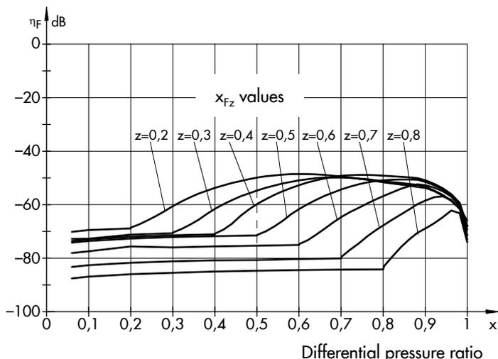
Diagram 2: Noise reduction with liquids depending on the differential pressure using flow dividers
