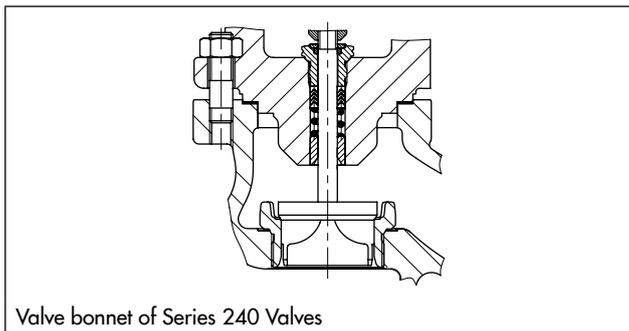
The temperature range of the standard packing is between  $-10$  and  $+220$  °C and can be extended by the use of an insulating section on the valve bonnet.
