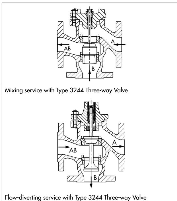
Mixing service with Type 3244 Three-way Valve
