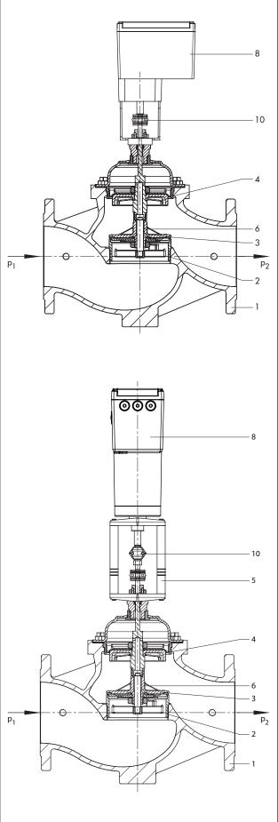
Fig. 2: Functional diagram of Type 3214 Globe Valve balanced by a diaphragm
