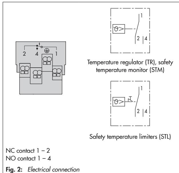
**Fig. 2:** Electrical connection
