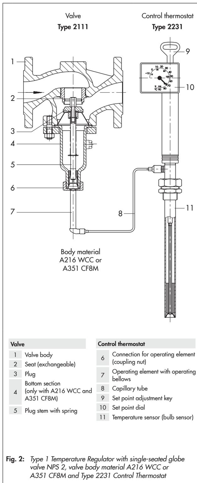
Fig. 2: Type 1 Temperature Regulator with single-seated globe valve NPS 2, valve body material A216 WCC or A351 CF8M and Type 2231 Control Thermostat
