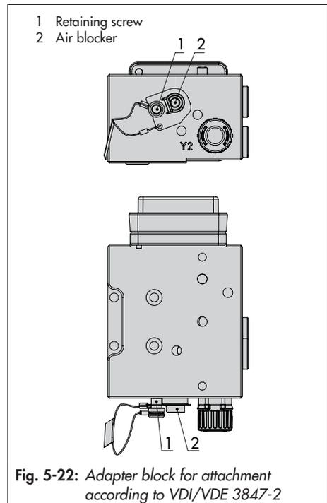
Fig. 5-22: Adapter block for attachment according to VDI/VDE 3847-2
