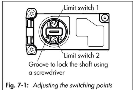
Fig. 7-1: Adjusting the switching points
