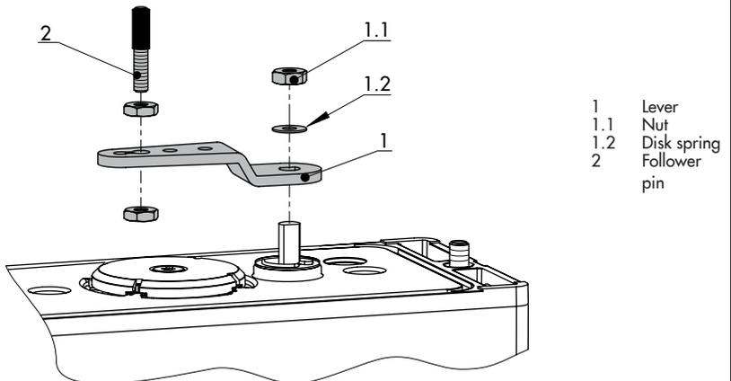
Fig. 5-4: Mounting the lever and follower pin
