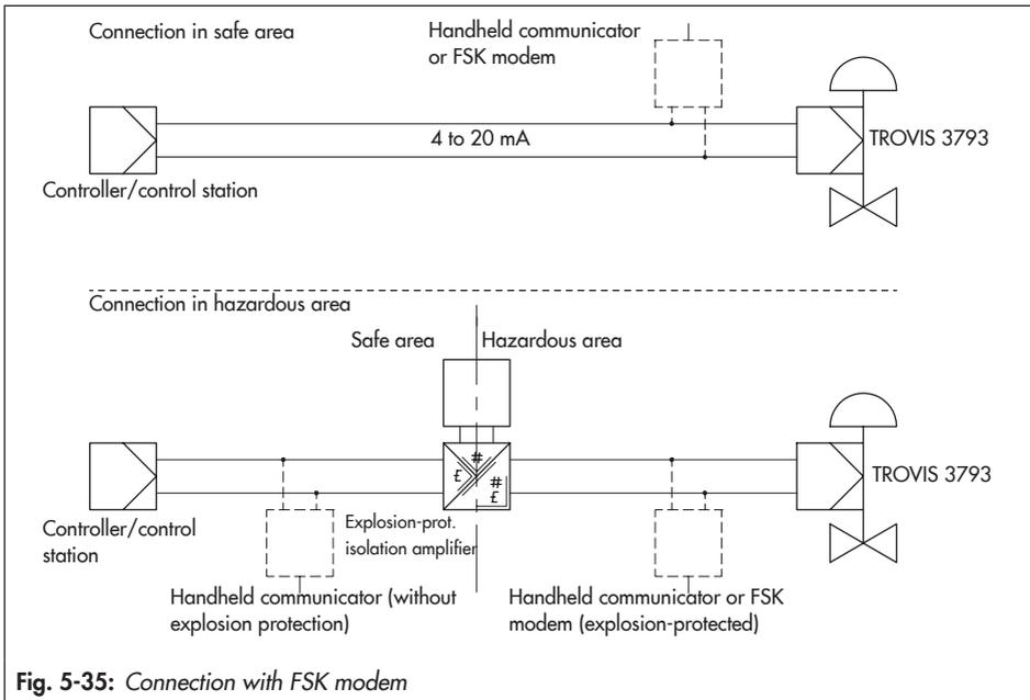
Fig. 5-35: Connection with FSK modem
