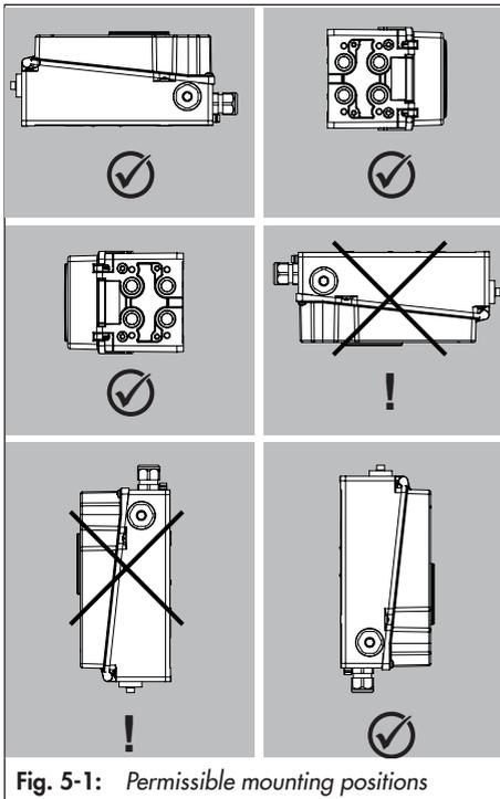
Fig. 5-1: Permissible mounting positions
