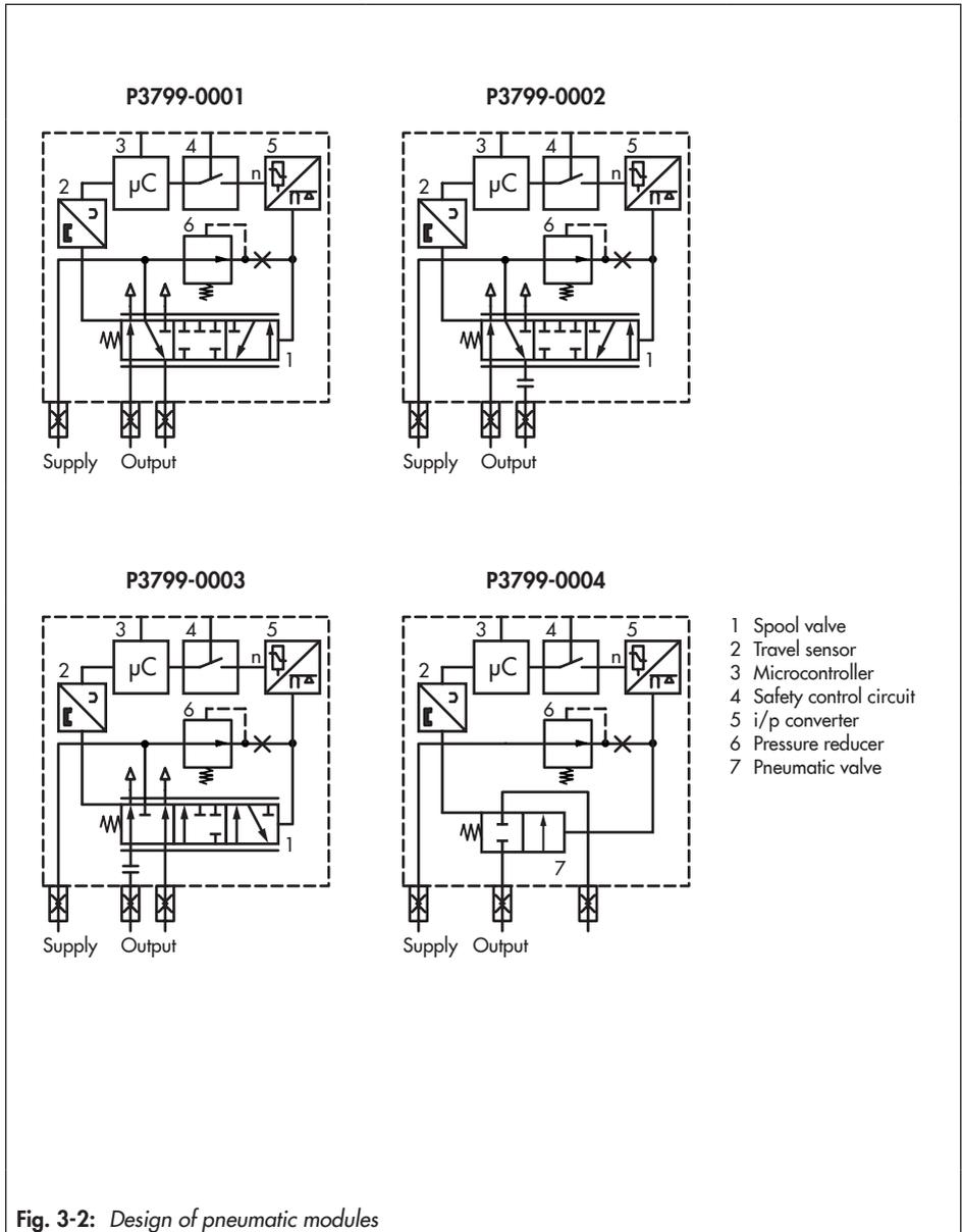
Fig. 3-2: Design of pneumatic modules
