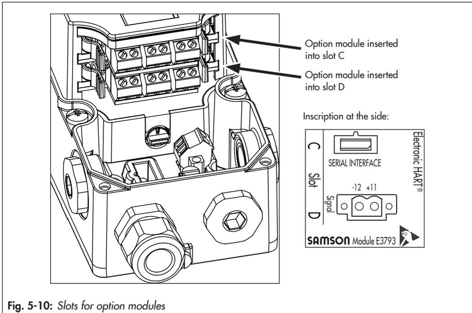
Fig. 5-10: Slots for option modules
