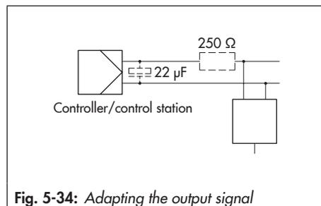
Fig. 5-34: Adapting the output signal
