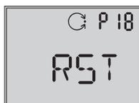
Press  $\ast$  and hold for six seconds. **6-5-4-3-2-1-** is counted down on the display.
