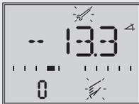
The wrench icon blinks on the display when the **positioner has not yet been initialized**. The reading indicates the lever position in degrees in relation to the mid-axis.
