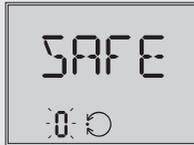
The valve moves to the fail-safe position.
