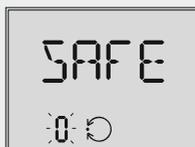
The valve moves to the fail-safe position.
