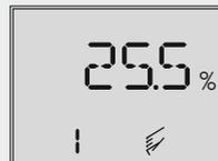
The positioner automatically returns to Code 0 if no settings are made within 120 seconds, but remains in the manual mode.
