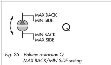
The volume restriction Q is used to adapt the air delivery to the size of the actuator:
