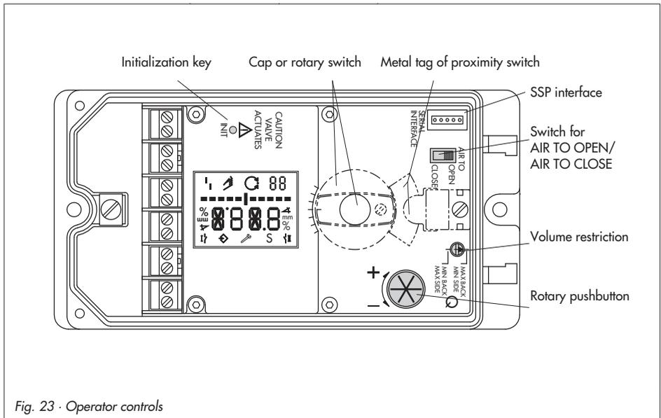
Fig. 23 · Operator controls
