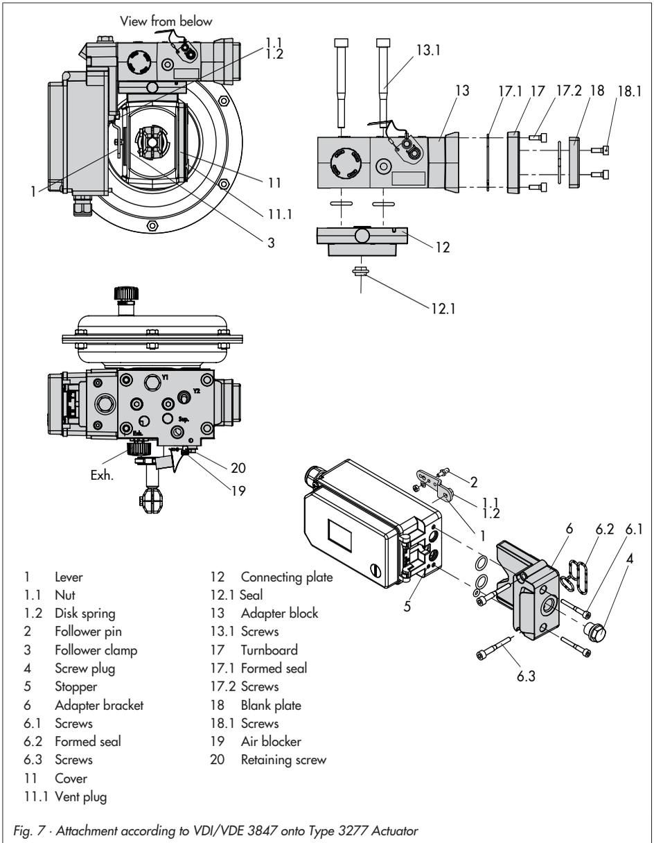
7. Insert screws (13.1) through the middle holes of the adapter block (13).
