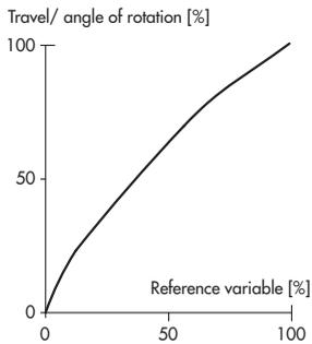
**VETEC rotary plug valve equal percentage**
