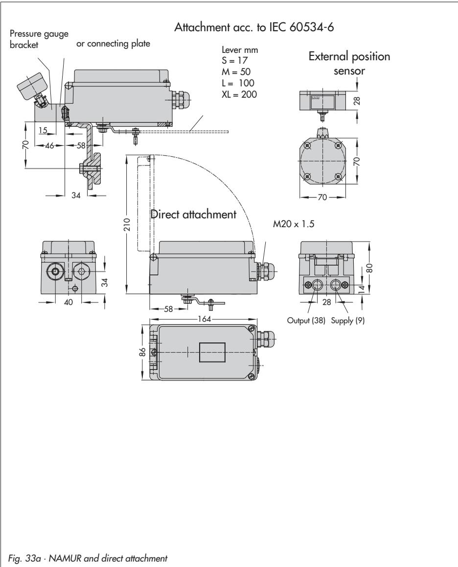
Fig. 33a · NAMUR and direct attachment
