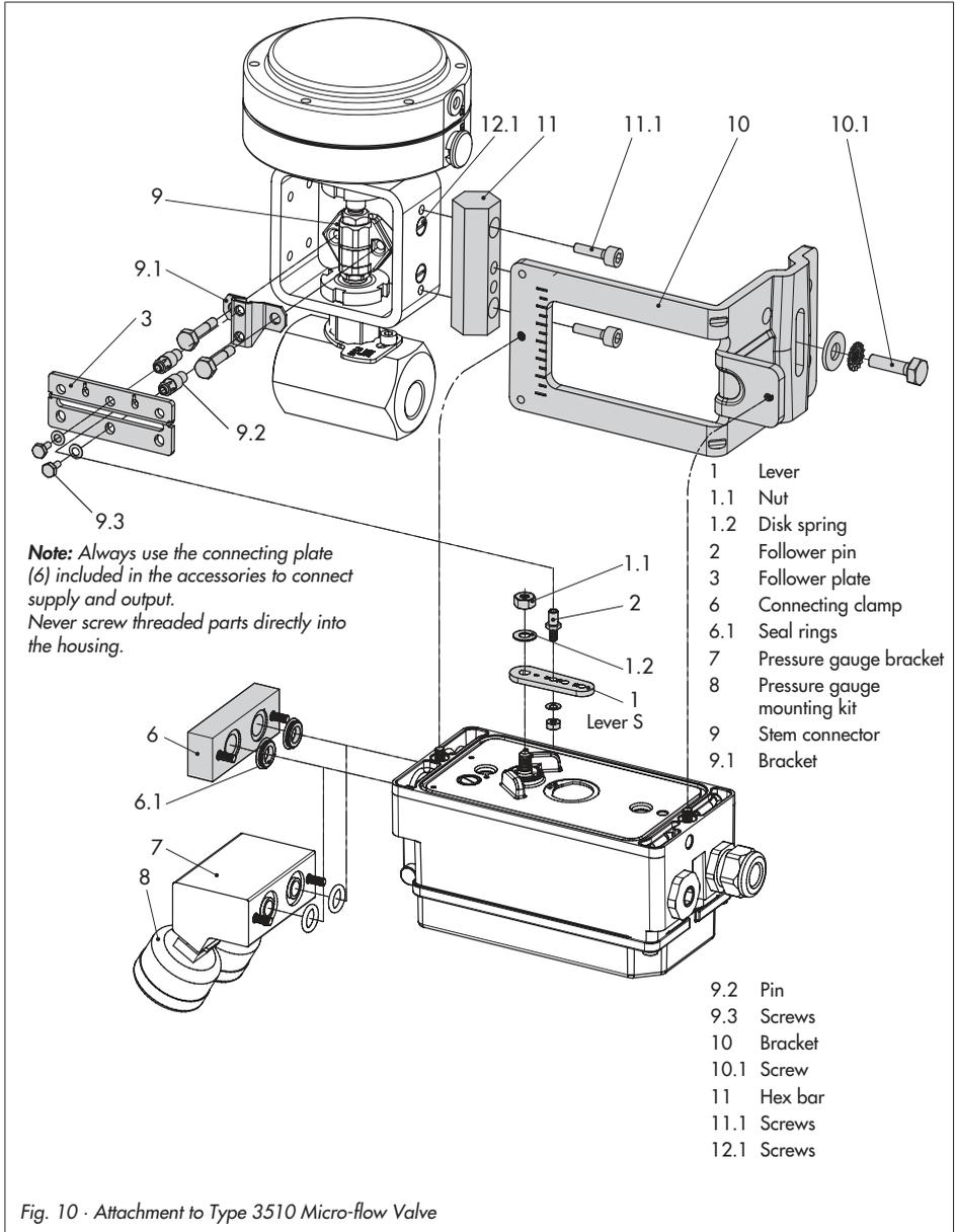
Fig. 10 · Attachment to Type 3510 Micro-flow Valve
