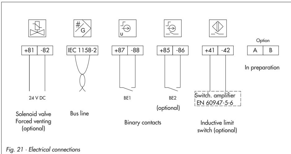
Fig. 21 · Electrical connections
