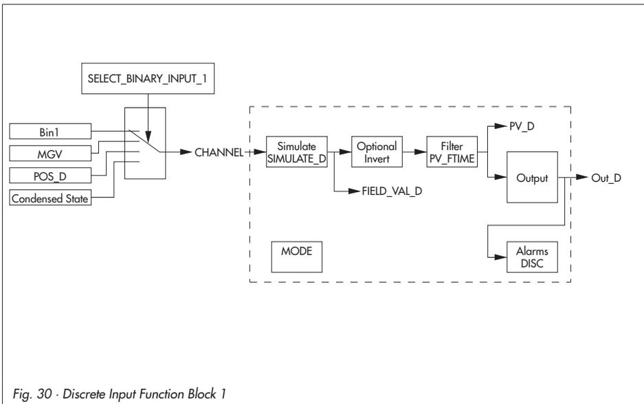
Fig. 30 · Discrete Input Function Block 1
