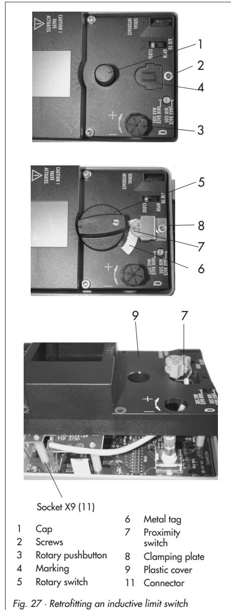
Fig. 27 · Retrofitting an inductive limit switch
