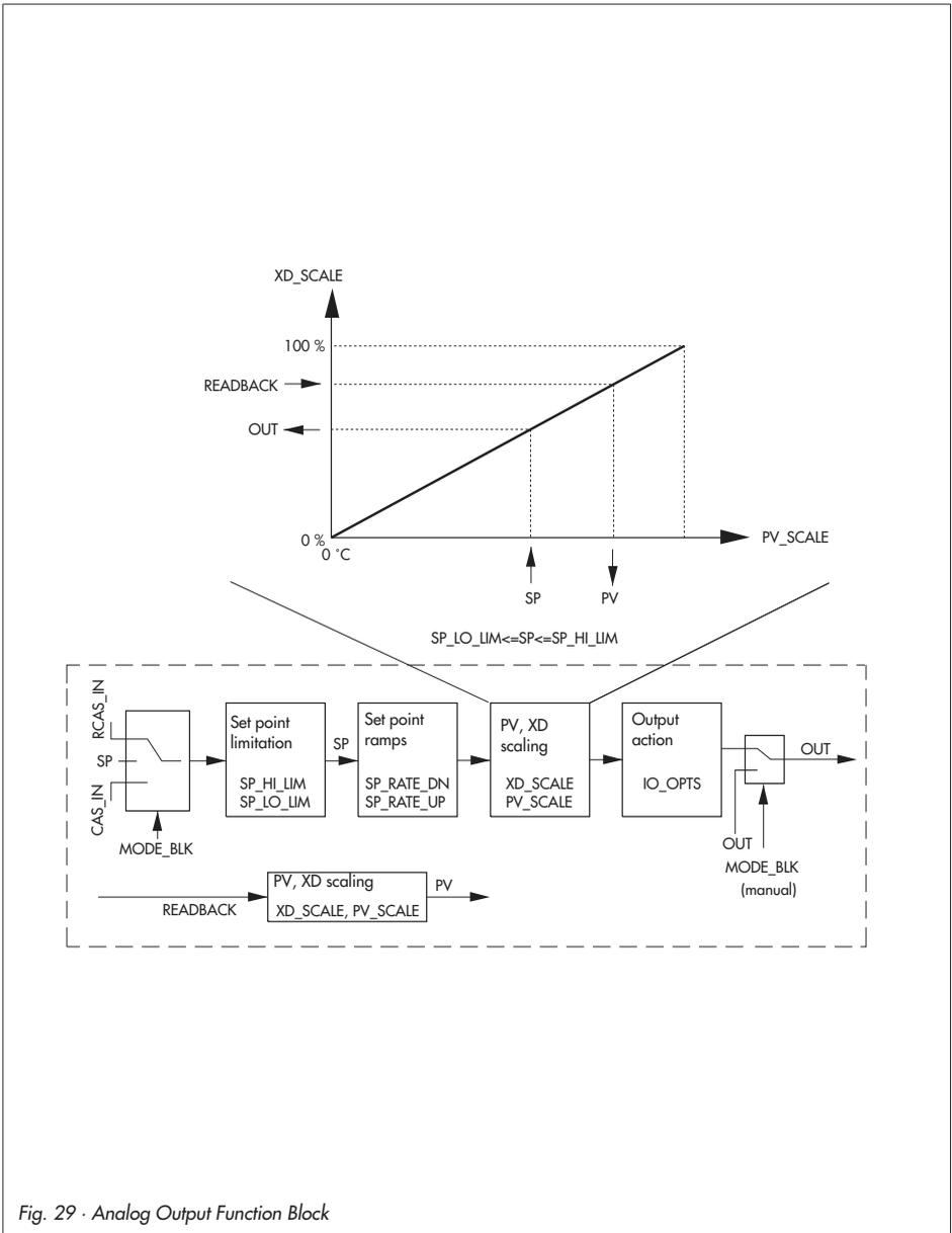
Fig. 29 · Analog Output Function Block
