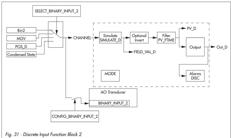
Fig. 31 · Discrete Input Function Block 2
