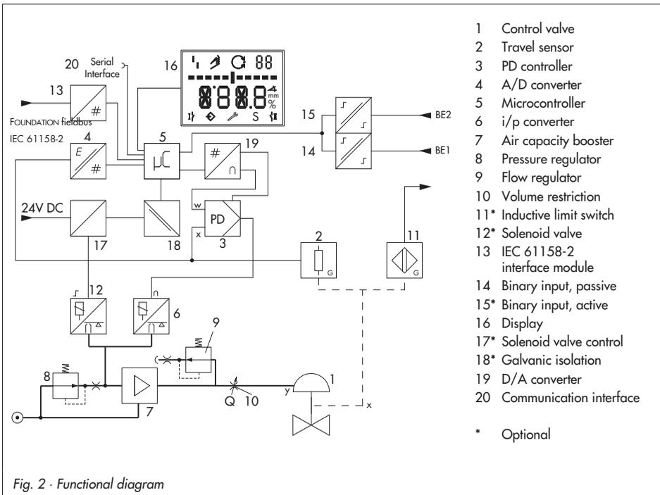
Fig. 2 · Functional diagram
