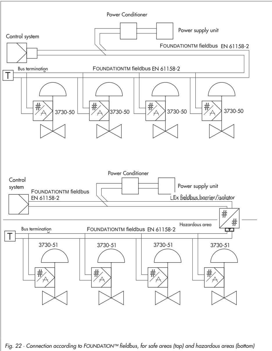
Fig. 22 · Connection according to FOUNDATION™ fieldbus, for safe areas (top) and hazardous areas (bottom)
