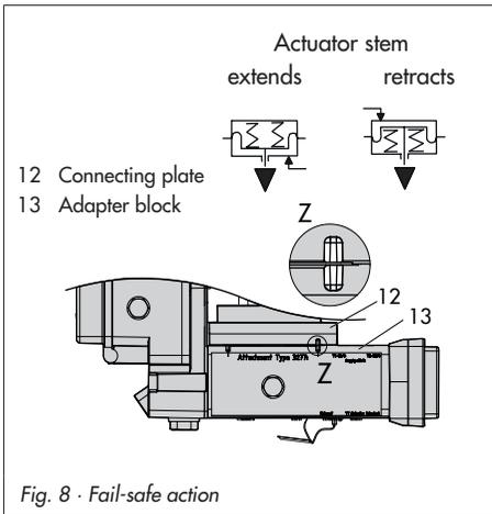
9. Mount the adapter block (13) together with the connecting plate (12) to the actuator using the screws (13.1).
