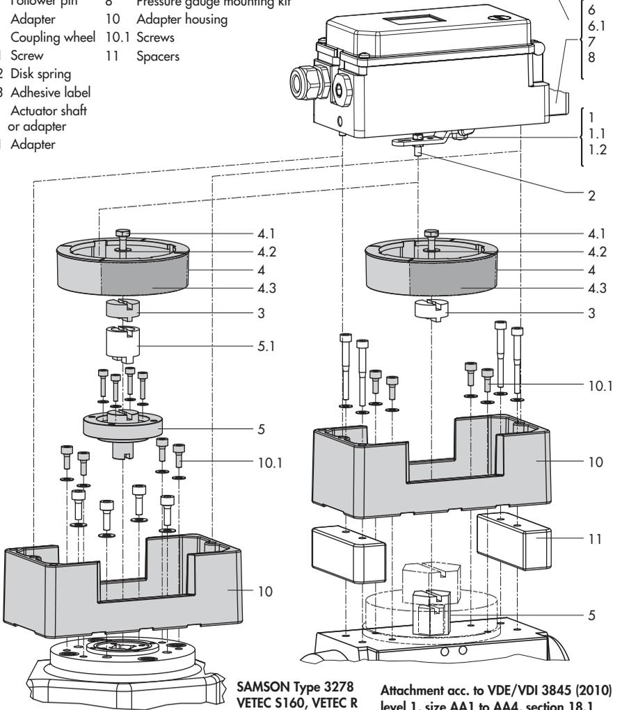
Fig. 14 · Attachment to rotary actuators (heavy-duty version)
