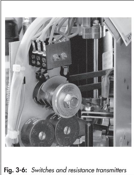
Fig. 3-6: Switches and resistance transmitters
