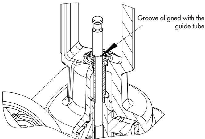
Fig. 10: Neutral position in automatic operation
