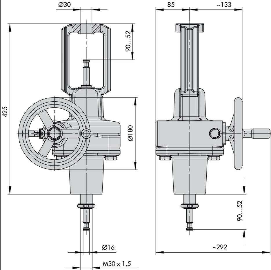
Dimensional drawings · Version with Ø 60 mm connection
