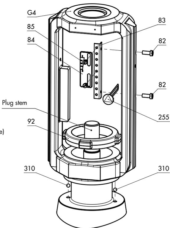
Fig. 7: Overview of yoke assembly with travel indicator scale in the standard version
