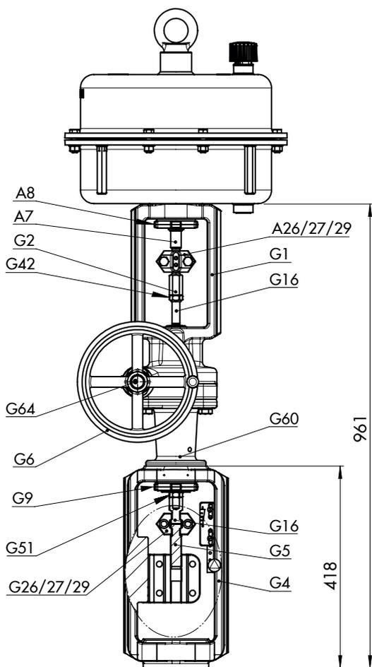
**Fig. 6:** Type 3273 Handwheel with 30 mm travel for mounting on Series 240 and 250 Valves with clamp-type anti-rotation fixture and Type 3271 Actuator with 1000 or 1400-60 cm<sup>2</sup> actuator area
