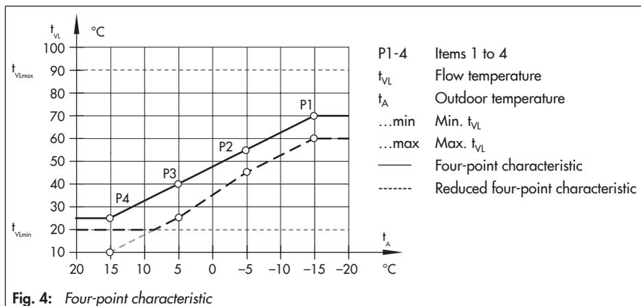
Fig. 4: Four-point characteristic
