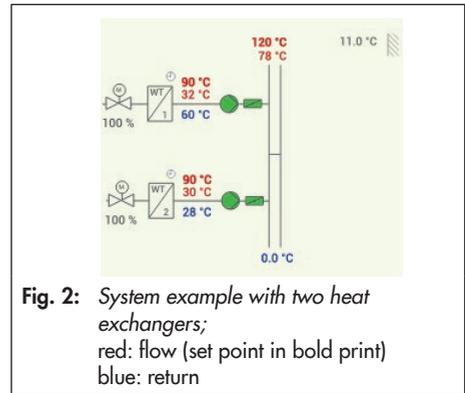
**Fig. 2:** System example with two heat exchangers;
