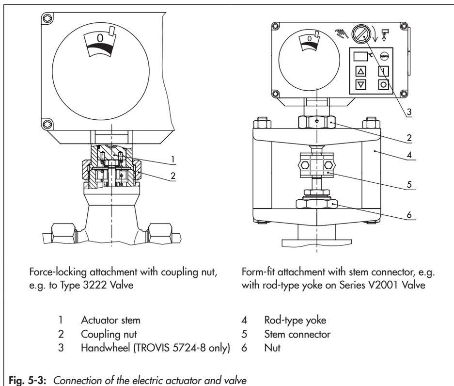
**Fig. 5-3:** Connection of the electric actuator and valve
