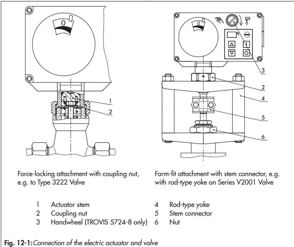
Fig. 12-1: Connection of the electric actuator and valve
