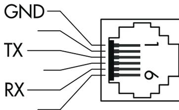
Fig. 5-4: Terminal assignment of RJ-12 jack
