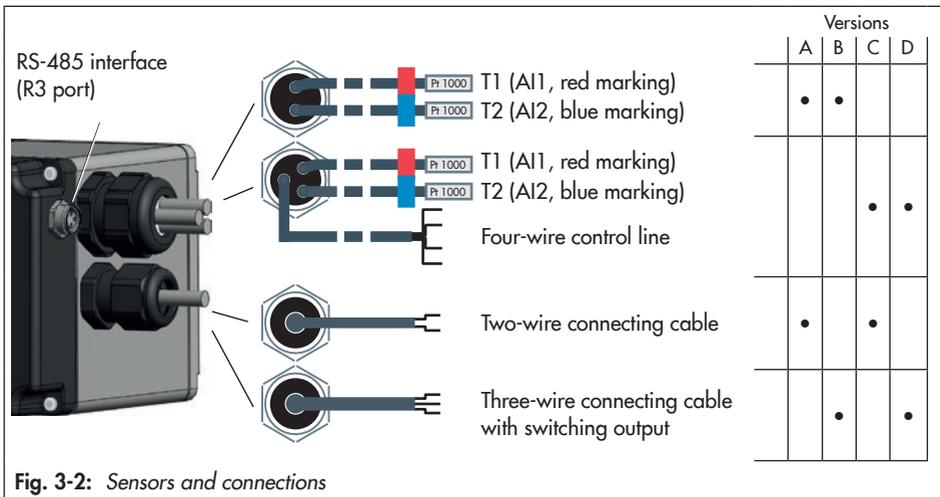
Fig. 3-2: Sensors and connections
