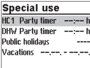
Turn the rotary switch to **#** (special times-of-use). The party timer for the first control circuit is now selected.
