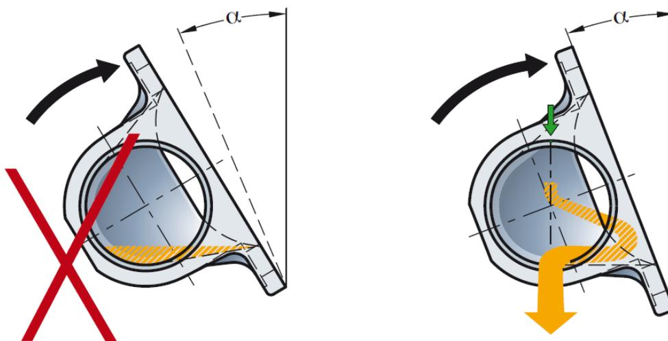
The individual self draining angle is marked on each valve body. The latest revision of the self draining angles is available on [www.sed-flowcontrol.com](http://www.sed-flowcontrol.com).
