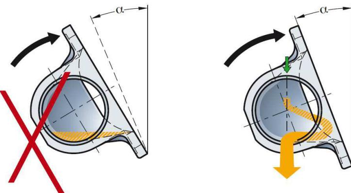
The individual self draining angle is marked on each valve body. The latest revision of the self draining angles is available on [www.sed-flowcontrol.com](http://www.sed-flowcontrol.com).
