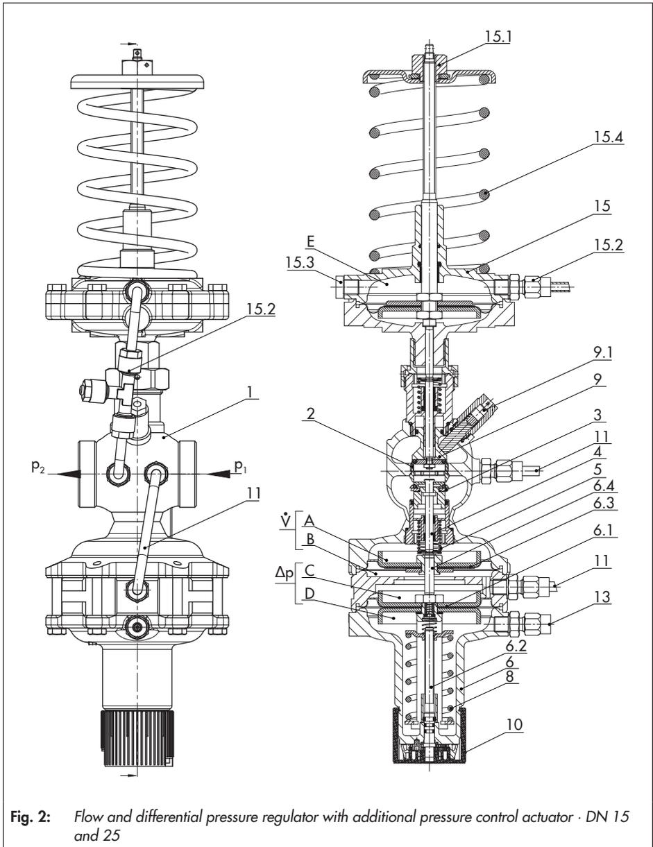
**Fig. 2:** Flow and differential pressure regulator with additional pressure control actuator · DN 15 and 25
