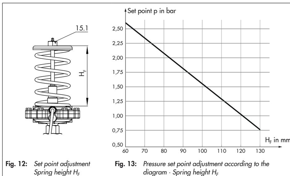
Fig. 12: Set point adjustment Spring height  $H_F$
