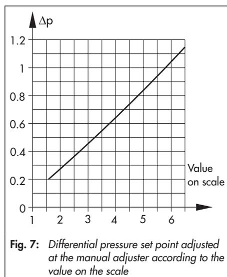
In this case, the set point can be directly adjusted at the manual adjuster (19) according to the scale.
