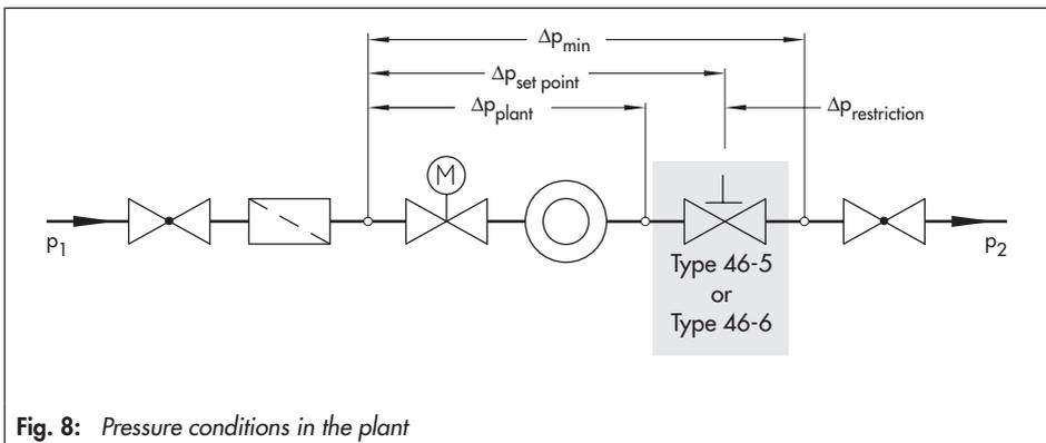
Fig. 8: Pressure conditions in the plant
