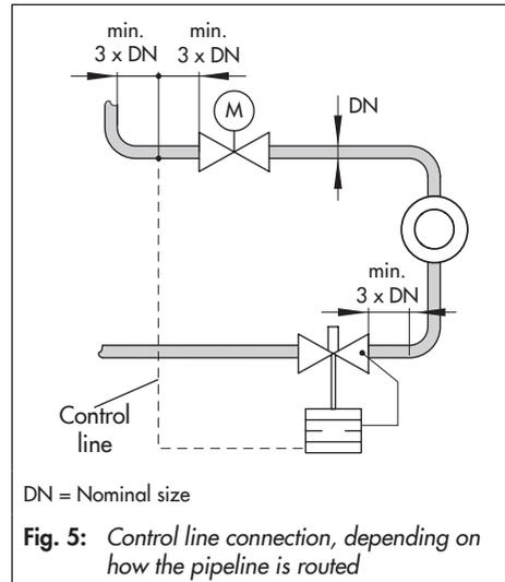
**Fig. 5:** Control line connection, depending on how the pipeline is routed
