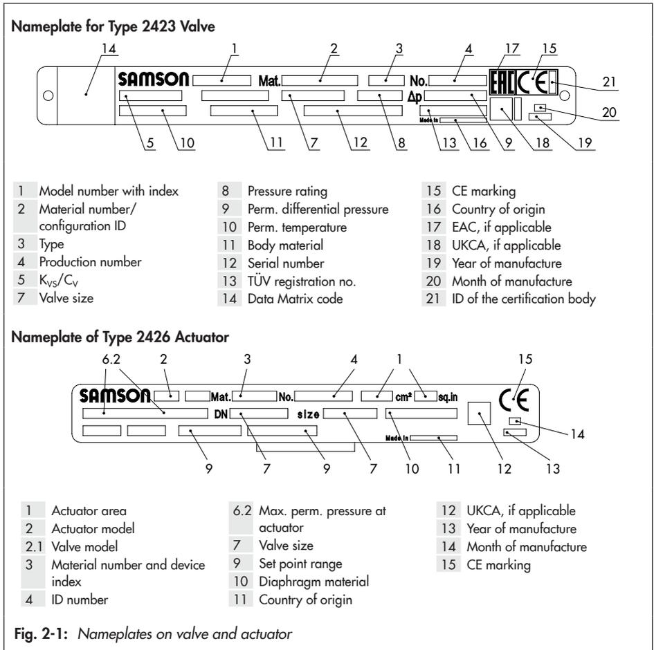
Fig. 2-1: Nameplates on valve and actuator
