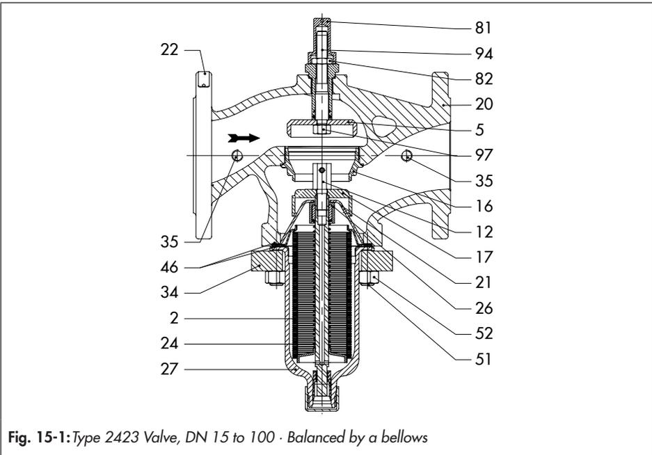
Fig. 15-1: Type 2423 Valve, DN 15 to 100 · Balanced by a bellows
