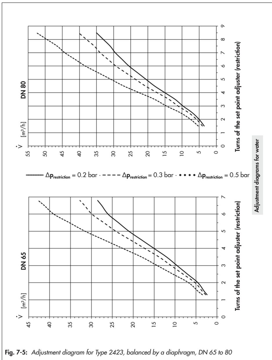
Fig. 7-5: Adjustment diagram for Type 2423, balanced by a diaphragm, DN 65 to 80
