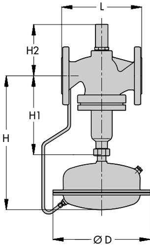
Type 2423 Valve, balanced by a diaphragm
