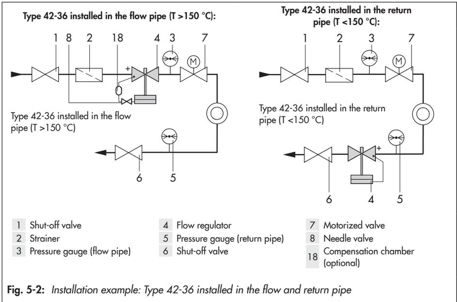
**Fig. 5-2: Installation example: Type 42-36 installed in the flow and return pipe**
