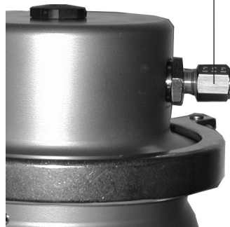
Fig. 5: Pneumatic set point adjustment
