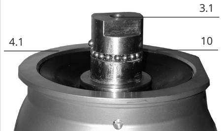
Actuator housing (10) with set point pressure port p_c and locking pin (16)
