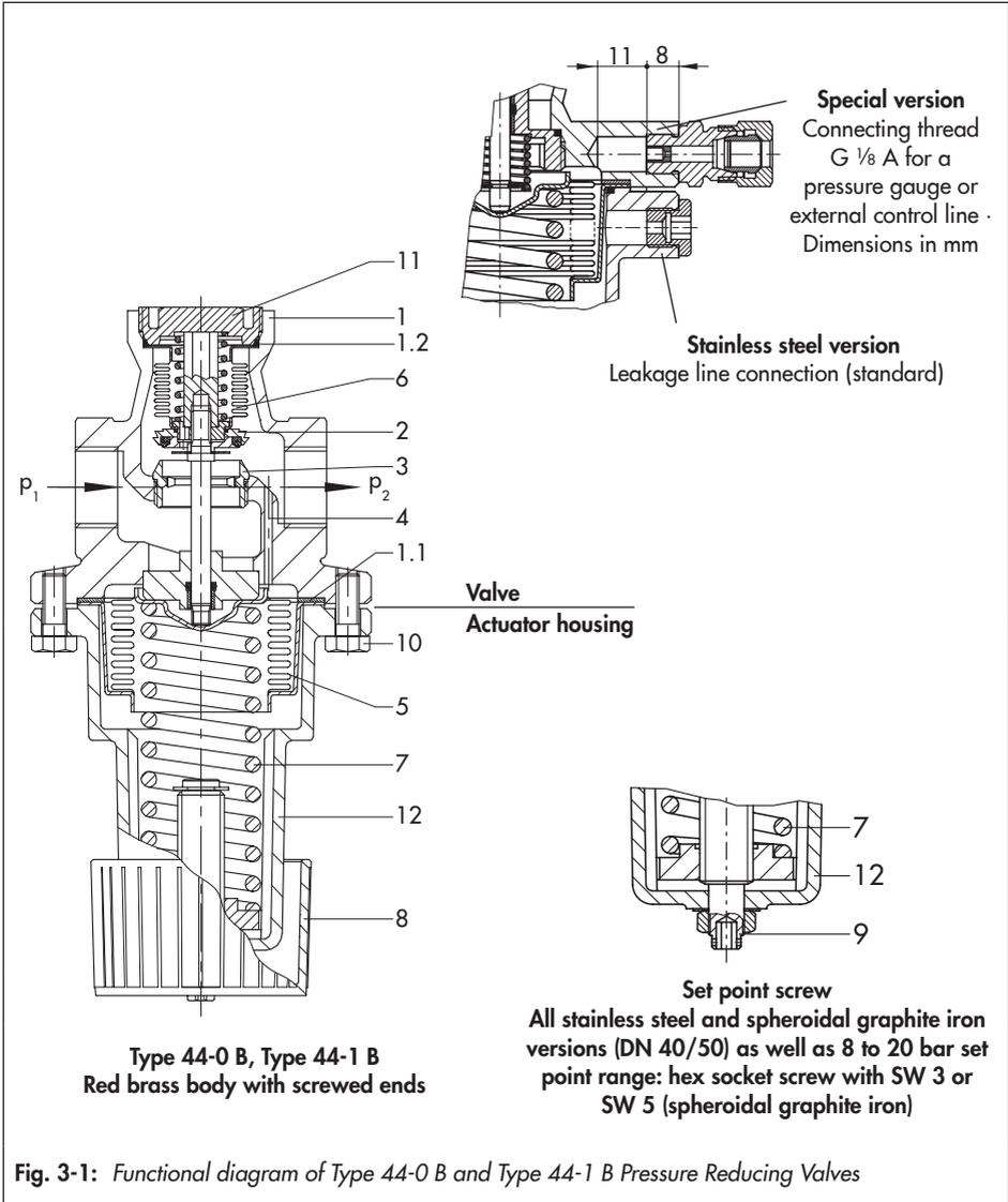
Fig. 3-1: Functional diagram of Type 44-0 B and Type 44-1 B Pressure Reducing Valves
