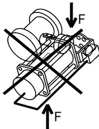
Make sure no improper forces act on the control line or accessories. Do not store the valve on the control line since this can cause damage.
