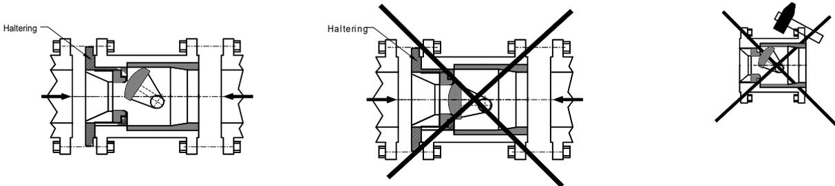
To ensure tight shut-off towards the atmosphere, cover the area between the armored bushing and the body with a sealing surface on both sides.
