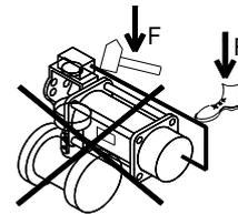
Do not step on the control line or accessories and do not damage them with tools.
