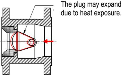
During the heating-up period, the heat is distributed rather unevenly across the valve. The components expand differently. As a result, the plug can get jammed in the seat ring (see drawing).
