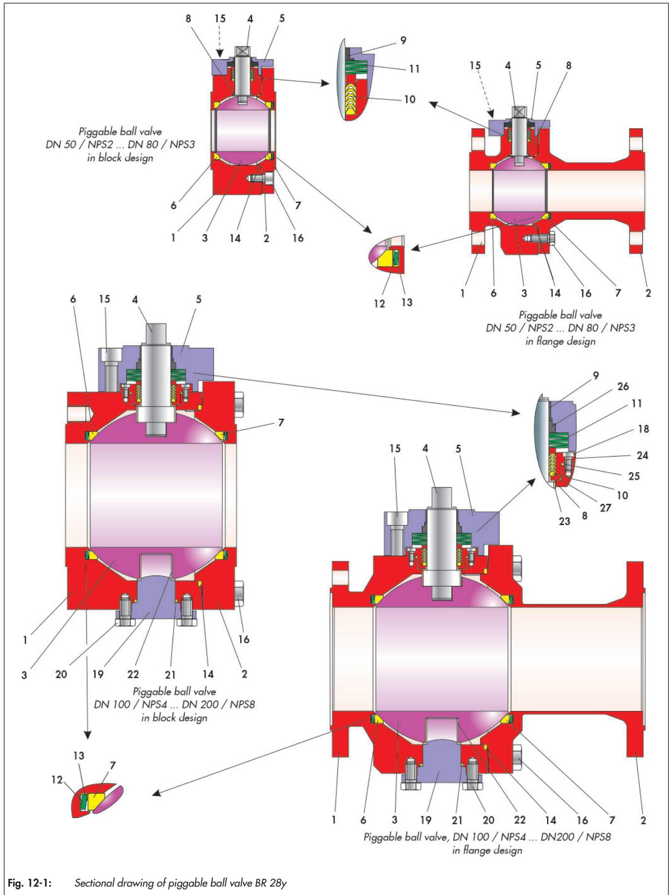
Fig. 12-1: Sectional drawing of piggable ball valve BR 28y
