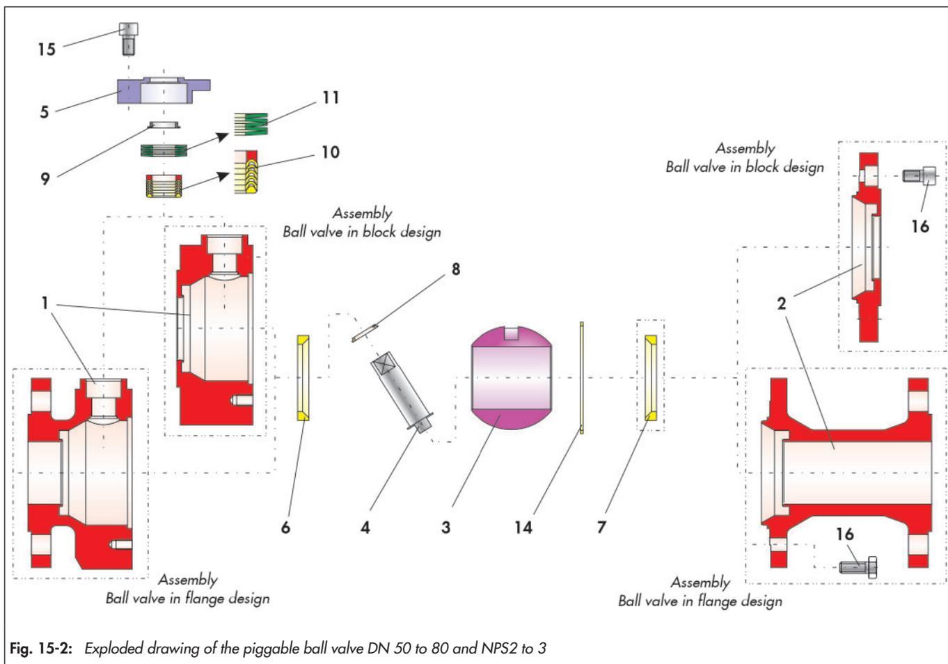
Fig. 15-2: Exploded drawing of the piggable ball valve DN 50 to 80 and NPS2 to 3
