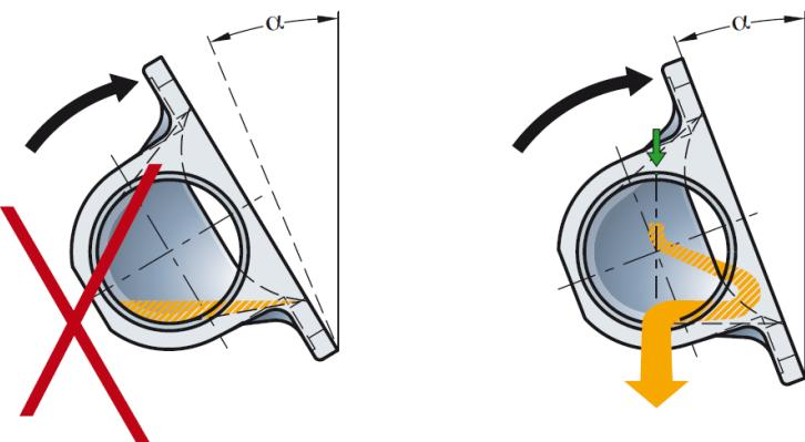
The individual self draining angle is marked on each valve body. The latest revision of the self draining angles is available on [sed.samsongroup.com](http://sed.samsongroup.com).
